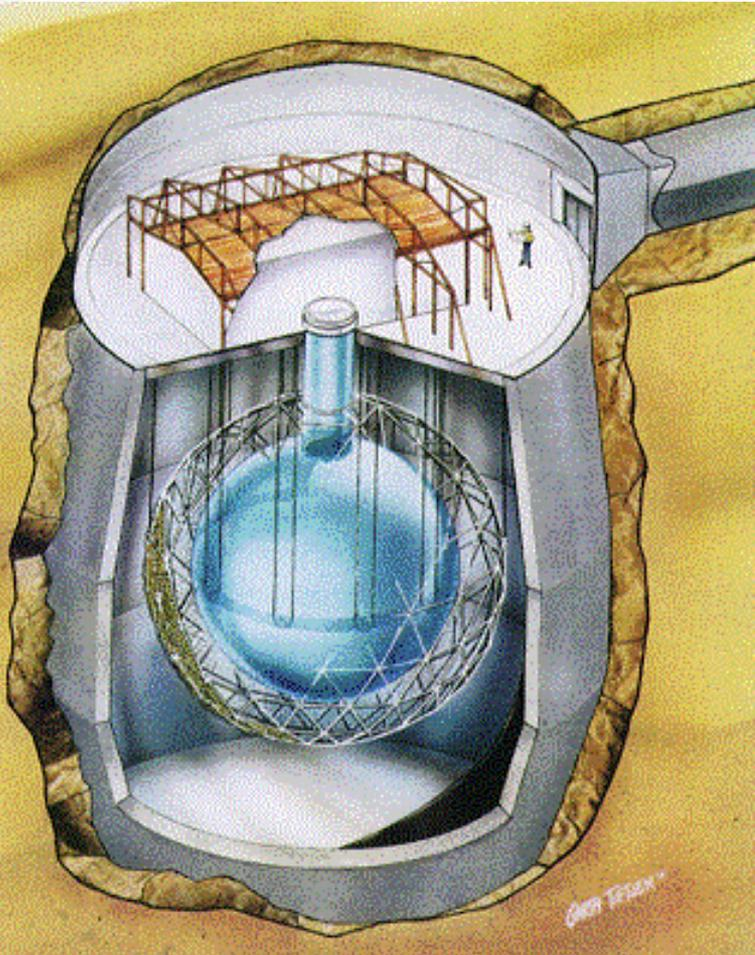
SNO: a real-time experiment detecting Cherenkov light emitted in 1000 tons of high purity **heavy water**  $D_2O$  contained in a 12 m diam. acrylic sphere, surrounded by 7800 tons of high purity water  $H_2O$
