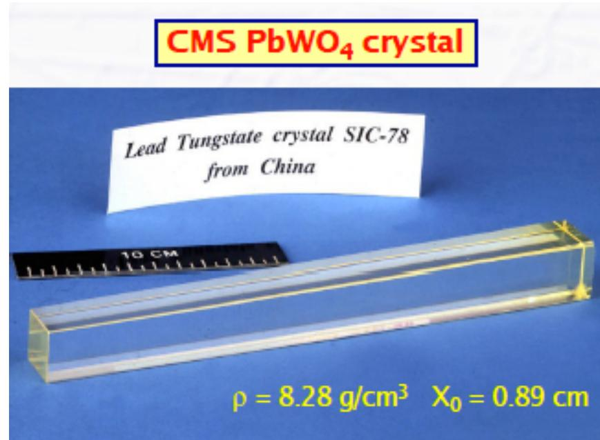
A  $\text{PbWO}_4$  crystal of the CMS electromagnetic calorimeter
