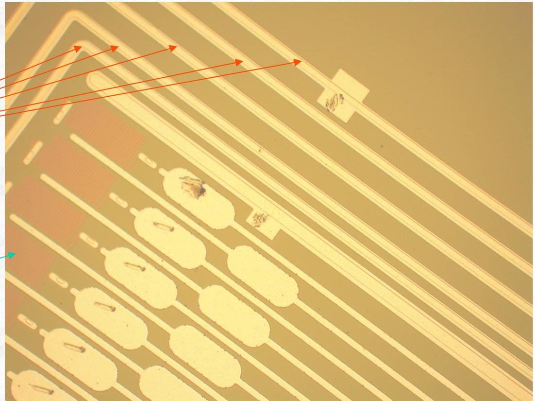
Example of a Si-detector with a single guard ring
