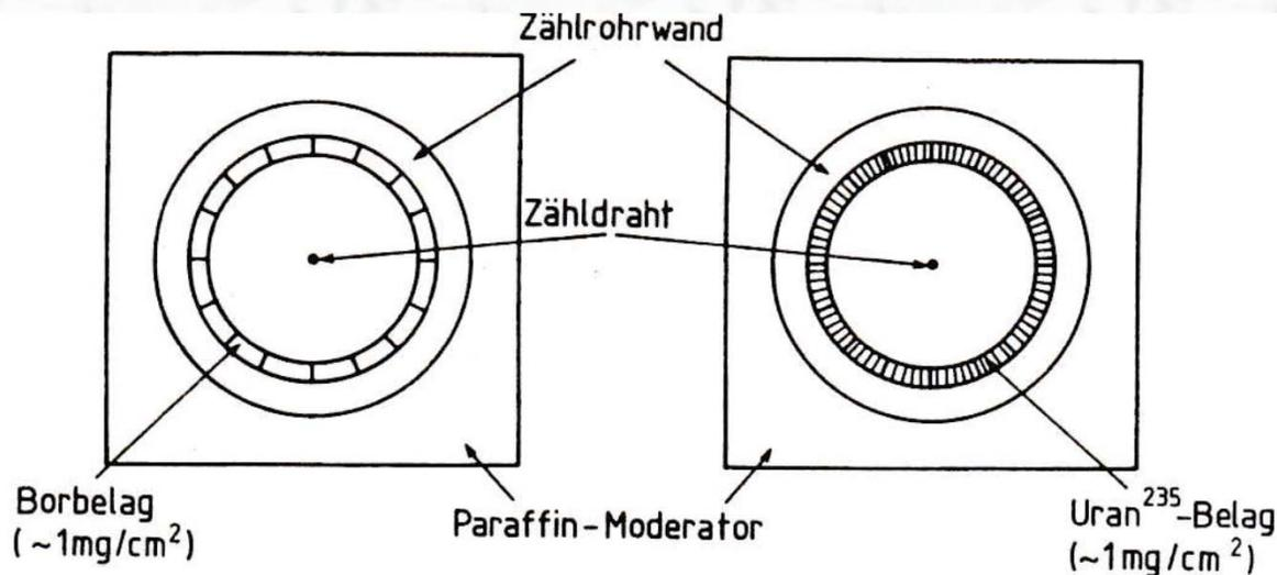
Principal method of neutron detection using ionisation counters (from Ref. [3])
