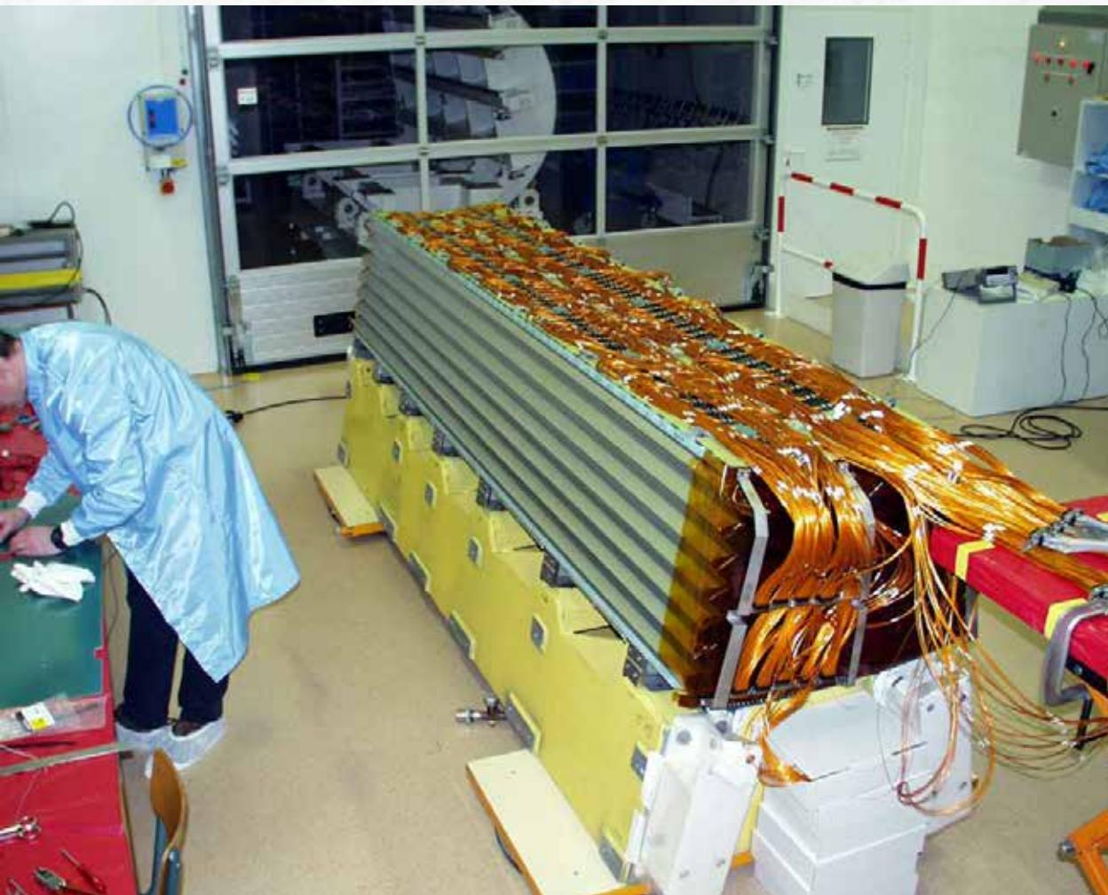
A slice of the ATLAS accordion barrel calorimeter, before installation;
