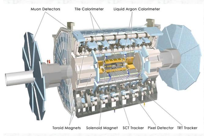
Solenoidal magnetic field (2T) in the central region (momentum measurement)
