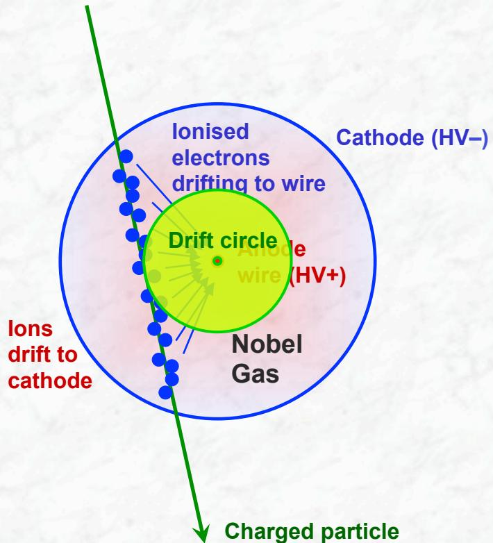
Example: muon in MDTs (**aligned !**)
