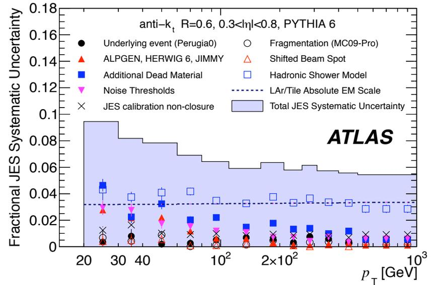
Fractional jet energy scale systematic uncertainty as a function of  $p_T$  for jets in the pseudorapidity region  $0.3 < |\eta| < 0.8$  in the barrel calorimeter. The total systematic uncertainty is shown as the solid light blue area. The individual sources are also shown, with statistical errors if applicable.
