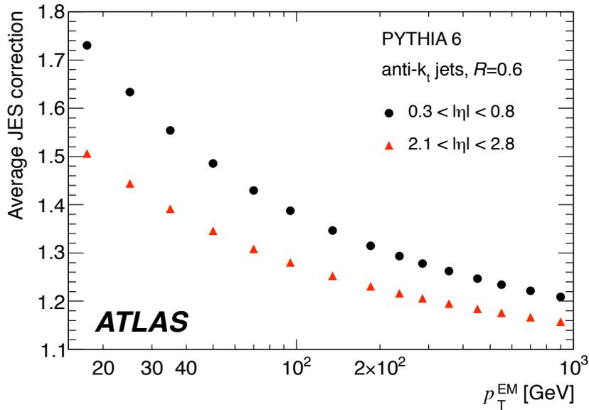
Average jet energy scale correction, evaluated using PYTHIA 6, as a function of jet transverse momentum at the EM scale for jets in the central barrel (black circles) and endcap (red triangles) regions, shown in EM scale  $p_T$  bins and  $\eta$  regions.
