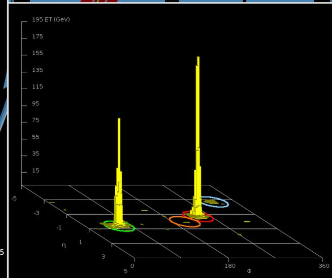
Event display that shows the highest-mass central dijet event collected during 2010, where the two leading jets have an invariant mass of 3.1 TeV. The two leading jets have  $(p_T, y)$  of (1.3 TeV, -0.68) and (1.2 TeV, 0.64), respectively. The missing  $E_T$  in the event is 46 GeV. From [ATLAS-CONF-2011-047](#).
