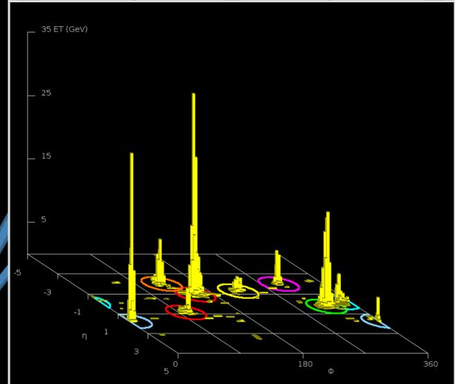
The highest jet multiplicity event collected by the end of October 2010, counting jets with  $p_T$  greater than 60 GeV: this event has eight. 1st jet (ordered by  $p_T$ ):  $p_T = 290$  GeV,  $\eta = -0.9$ ,  $\phi = 2.7$ ; 2nd jet:  $p_T = 220$  GeV,  $\eta = 0.3$ ,  $\phi = -0.7$  Missing  $E_T = 21$  GeV,  $\phi = -1.9$ , Sum  $E_T = 890$  GeV. The event was collected on 5 October 2010.
