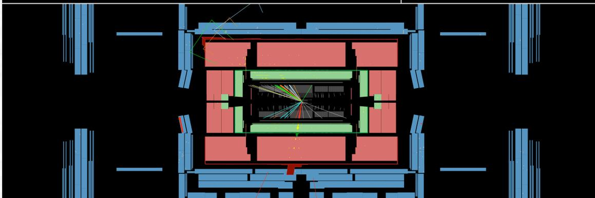
A display of the reconstructed event with the highest  $m_{\text{eff}}$  (1548 GeV) found in the ATLAS data sample. This event possesses four jets with  $p_{\text{T}} > 40$  GeV ( $p_{\text{T}} = 636, 189, 96$  and 81 GeV respectively) and  $E_{\text{T}}^{\text{miss}} = 547$  GeV.
