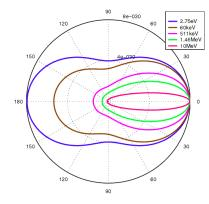
Figure 1: The angular dependence of the Klein-Nishina cross-section for a range of energies.
