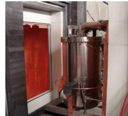
The XENON100 detector in its low-background shield at LNGS
